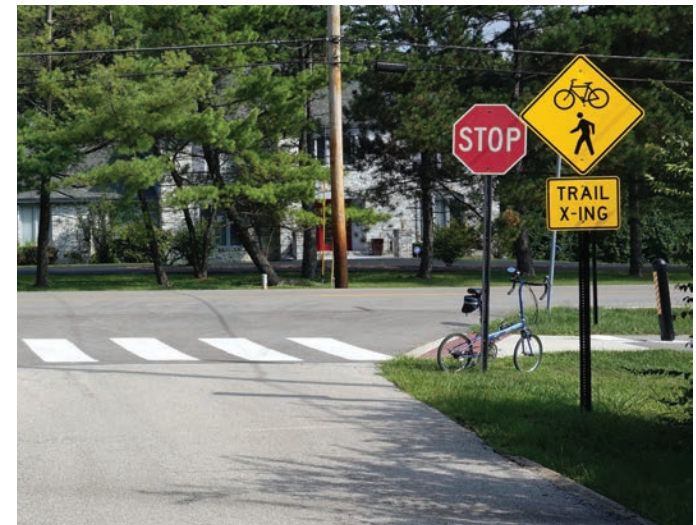
Sidepath Advisory Signs. Top: Variation of the MUTCD’s Railroad Advance Warning Sign, modified as a sidepath advisory. This sign should be used on both sides of a road with sidepaths. This installation is on Speer Boulevard in Denver, advising of the parallel Cherry Creek Trail. Florida DOT advises a similar sign. Below: Trail crossing advisory sign on an intersecting side street, installed on Clayton Road in suburban Saint Louis.
