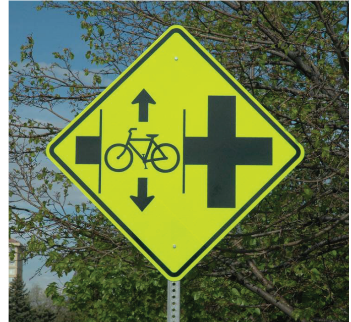
Sidepath Advisory Signs. Top: Variation of the MUTCD’s Railroad Advance Warning Sign, modified as a sidepath advisory. This sign should be used on both sides of a road with sidepaths. This installation is on Speer Boulevard in Denver, advising of the parallel Cherry Creek Trail. Florida DOT advises a similar sign. Below: Trail crossing advisory sign on an intersecting side street, installed on Clayton Road in suburban Saint Louis.
