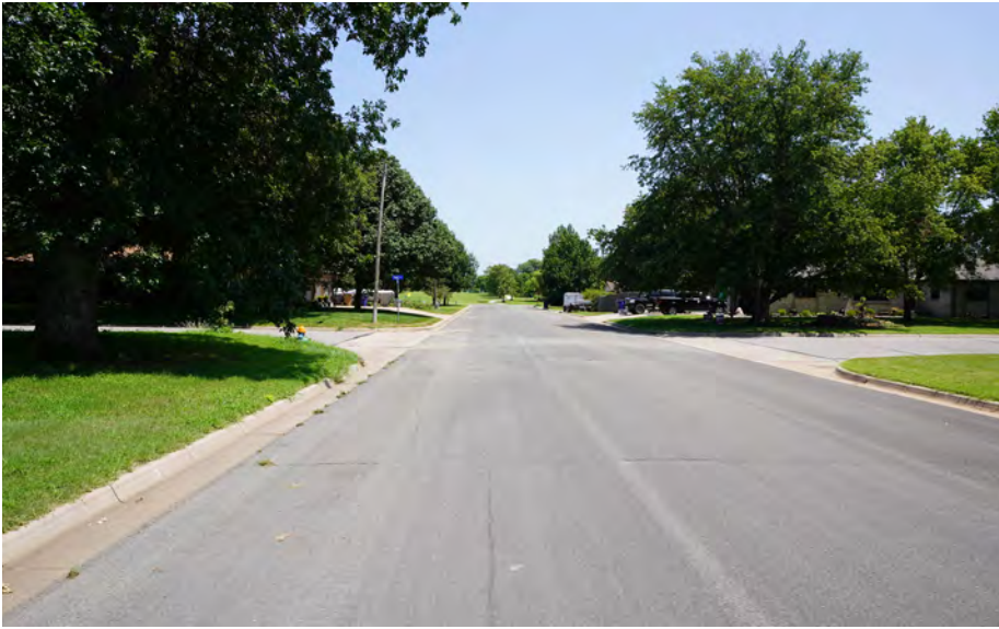
16 / Many of Clearwater's streets (like Park Ave shown here) are close to 40' wide.
